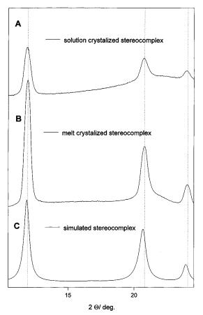
Figure 2. Experimental powder pattern of solution (A) and melt-crystallized (B) stereocomplexes and the simulated powder pattern of the calculated stereocomplex (C).
