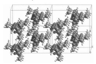
**Figure 4.** Simulated crystal structure of  $\beta$ -PLLA (- - -, van der Waals contacts).
