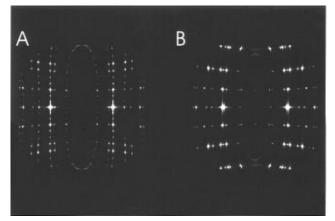
**Figure 6.** Simulated fiber pattern of  $\alpha$ -PLLA (A) and  $\beta$ -PLLA
