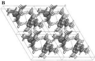
**Figure 3.** Simulated crystal structure of the stereocomplex (---, van der Waals contacts) with parallel orientation of the helices (A) and antiparallel orientation of the helices (B).
