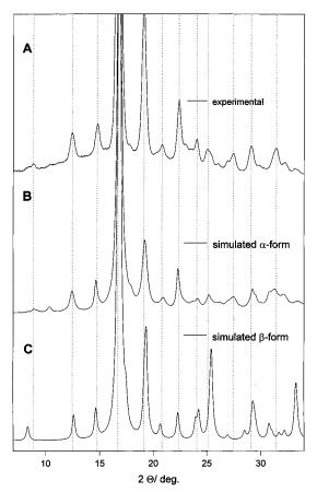
Figure 1. Experimental powder pattern of PLLA (A) and simulated powder patterns of calculated α-PLLA (B) and  $\beta$ -PLLA (C).
