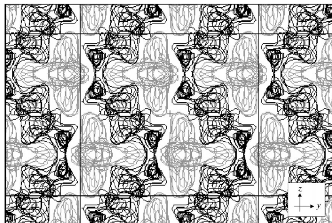
Figure 12 FAM phased synthesis in the projection along the x axis. Black contours correspond to the high-density region and grey contours to the low-density region.
